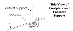
FIGURE 6.10 Angle Adjustment
